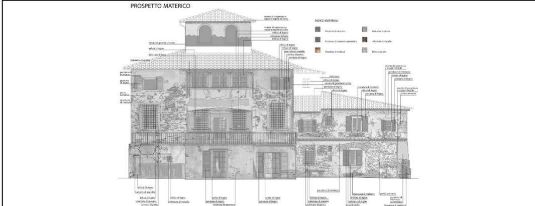
**Figure 3.** Ortho images for thematic maps for material analysis (Restoration Lab. 2014).
