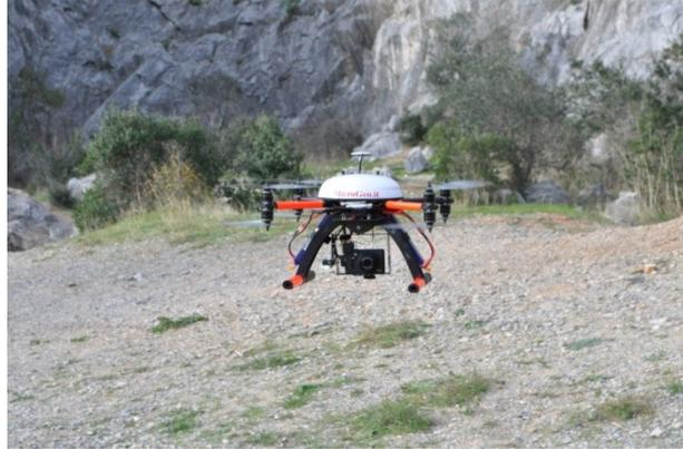
Figure 2 - Optocopter AeroMax 800 tested by Lab. GeCo for a digital photogrammetric project
