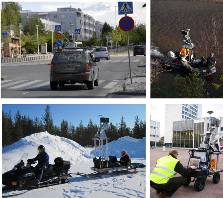
Figure 3 -Different vehicles for Mobile Mapping Systems (from:
