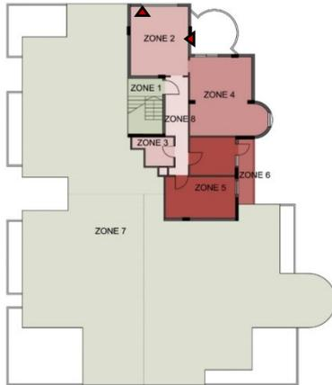
Figure 11 Zonings of the flat including location of indoor & outdoor Hobo data loggers
