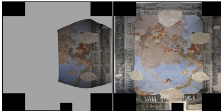
Figure 5: Partial UV map of a single photogram (left) and total overall UV map (right)
