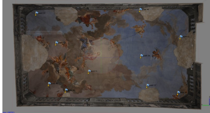
Figure 7: Laser scanner model textured via SfM software
