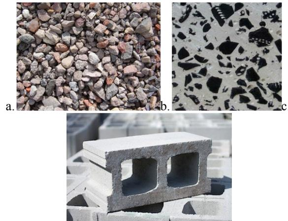
Figure 10: a. Recycled aggregates, b. Concrete with rubber pieces, c. CO<sub>2</sub> cured concrete masonry blocks [29-31]
