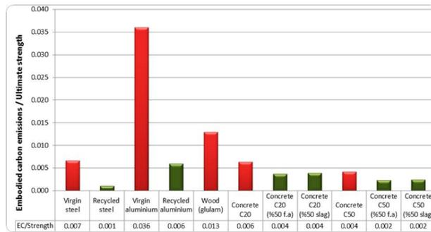
Figure 9: Embodied carbon emissions to strength ratios in structural materials (Kuruscu and Girgin 2014)
