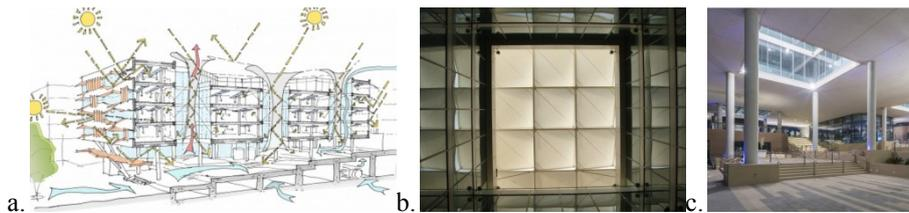
Figure 3: a. Sketch of ventilation and Venturi effect in Siemens HQ (UAE, 2013), b. Orientation of voids for Venturi effect, c. A typical exterior shaft [14, 15]
