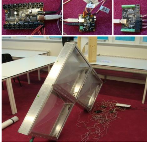
Fig 10. The finished skin as an assembly of three interactive components with built-in micro-controllers and sensing (proximity, touch and light- above) and actuation systems per component.
