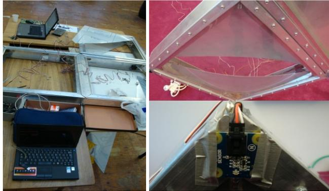
Fig 09. View showing the assembly details of the actuators and motors on the internal frame of the prototype and the mounting of touch sensors on the external frame of the prototype.
