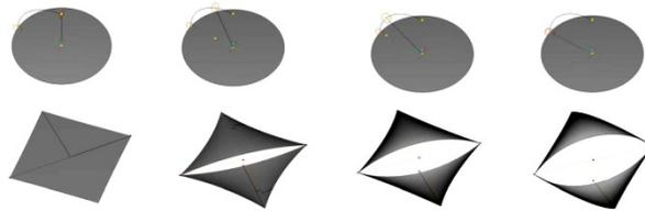
Fig 07. The Generative Components based simulation showing the first row with different sun directions and the second row representing various opening configurations of the PET flaps.
