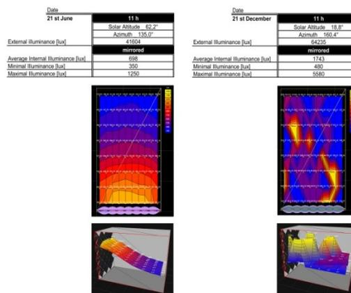
Fig 11. An example image of the extensive analysis showing the results of the daylight analysis on the 21st June and 21st December at 11 a.m.
