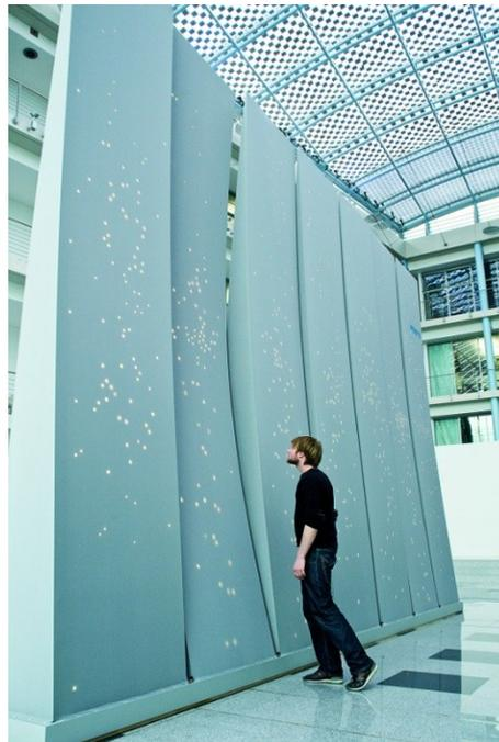
Fig 01. The skin of each InteractiveWall covered by a unique, irregular distribution of dynamically controlled LED's that form a highly reactive interface.
