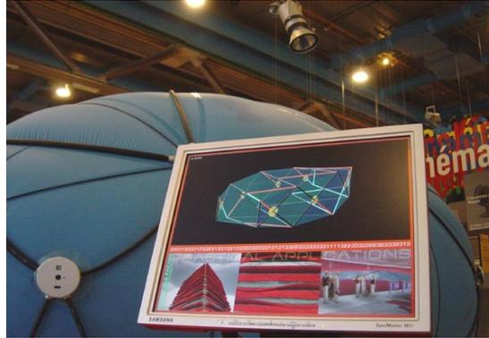
Fig 05. The NSA Muscle's real-time computational process being shown via a monitor at the NSA exhibition. The activity of the physical muscles is displayed in the digital world in real-time in three colors in the model: red / inflating state, blue / deflating state, and gray / passive state, and in the internally used organizational 72 digit string.
