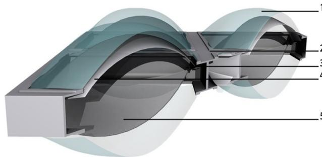
Fig 08. View showing the internal structural make-up of the sandwich component. The ETFE sheets (1) are inflated and connected to the C profiles (2) along their perimeter. The pointer (3) shows the connection point between one of the movable extremities and the small rail in aluminium (that is welded to the C profile). The two movable membranes (4, 5) have a triangular shape and assume two opposite curvatures during their movement.
