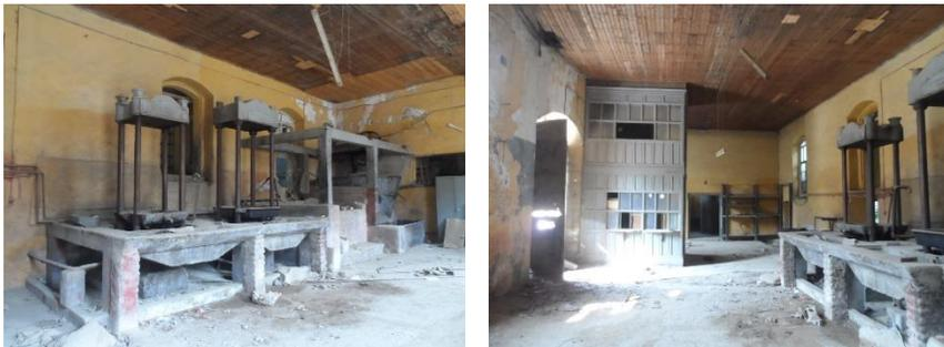
Figure 9-10. The olive oil workshop - mill stone, hydraulic presses, office.
