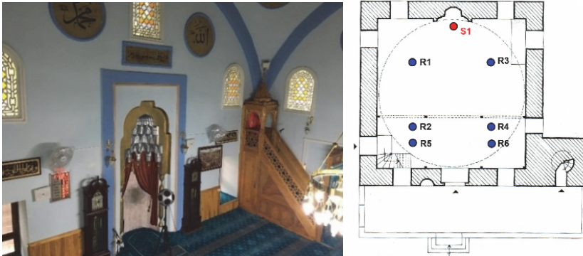
Figure 2. Interior view of Hüsrev Ağa Mosque and positions of sound source (S) and receiver points (main worship area; R1, R2, R3, R4 upper floor for women; R5, R6)
