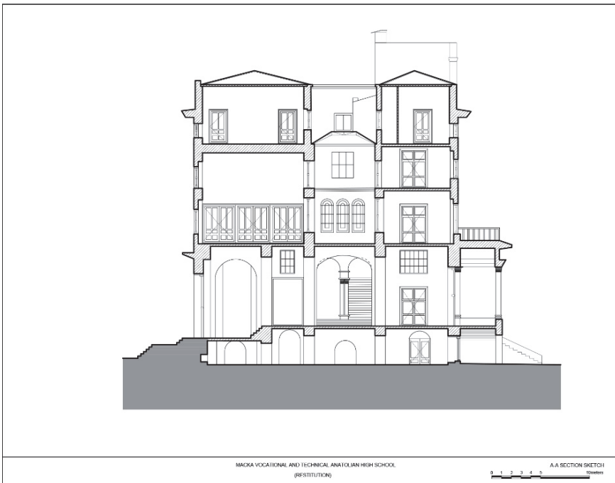
Sketch 3: A-A section sketch; survey-restitution.
