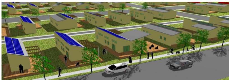
Figure 9. An urban design study testing the density of housing development with roof-mounted PV arrays. The density can be considerably higher than the solution shown
