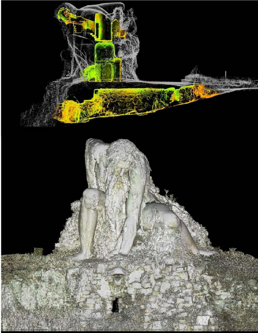
Figure 6. The Giant of the Appennino. Orthoimages of the point cloud showing the inner rooms and the main elevation.
