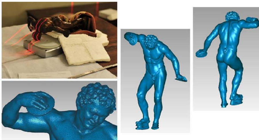
Figure 4. 3D digitization of a bronze statuette representing a Dancing faun with cymbals , first quarter of the 18 th century (Museum of Casa Martelli): a picture taken during the survey by means of a multistripe laser triangulation scanner, and the digital 3D model shown without the photographic texture.
