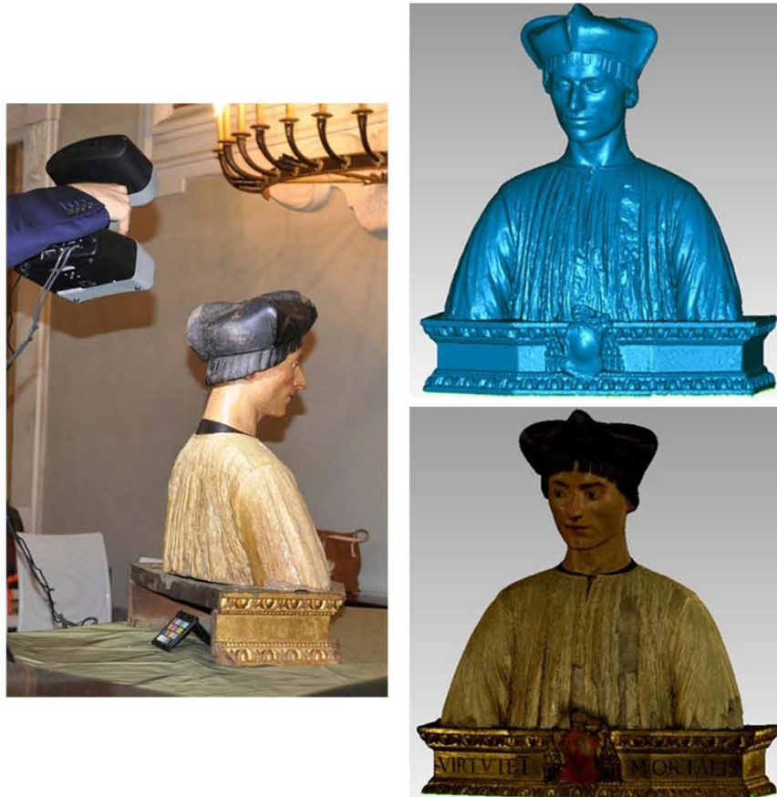
Figure 5. 3D digitization of the bust portrait of Ugolino Martelli, 1518-1519 (Museum of Casa Martelli): a picture taken during the survey by means of a hand-held scanner, and, on the right, the digital 3D model shown without and with the photographic texture.
