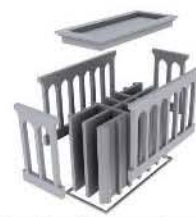
Figure 8. 3D model of badgir opening and blade
