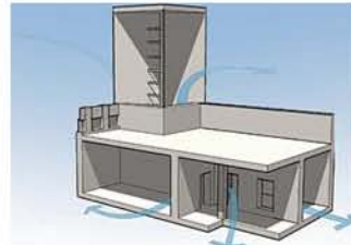
Figure 2. Air convection in Badgir
