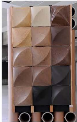
Figure 3. TraShell™ from rice straw, organic ash and bio-resin.
