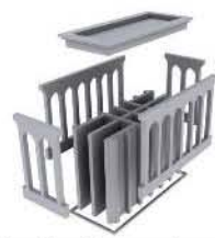
Figure 8. 3D model of badgir opening and blade
