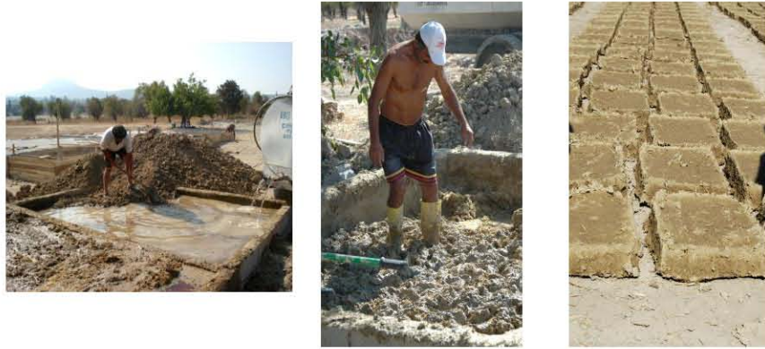
Figure 7. Preparation of mud brick [Özbekoğlu 2008]
