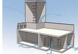
Figure 2. Air convection in Badgir
